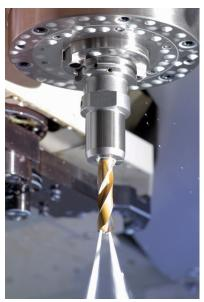
orders, and makes a company less competitive. Coolant that is not efficiently applied to the cutting zone is a leading contributor to these problems. The good news is that the situation can be corrected through proper application of high pressure coolant.
